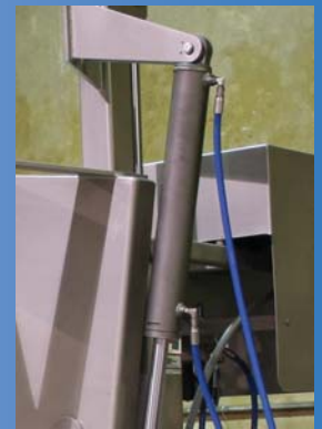
The EasyPicker utilizes stainless steel hydraulic fittings
