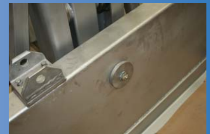
The EasyPicker features a heavy-duty pivot bolt that allows the carriage to rotate up to 100 degrees.
