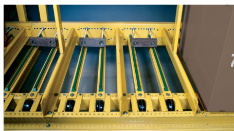
Battery compartment with adjustable back stop.
