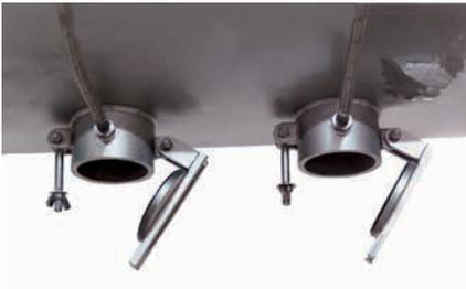
Low velocity steam injectors with quick opening cover for sanitation.
