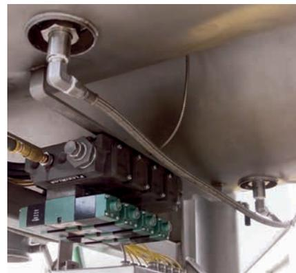
Quick disconnect direct steam injector.
