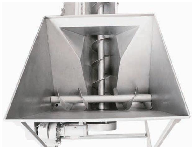
Inside hopper, showing feed screw and metering screw
