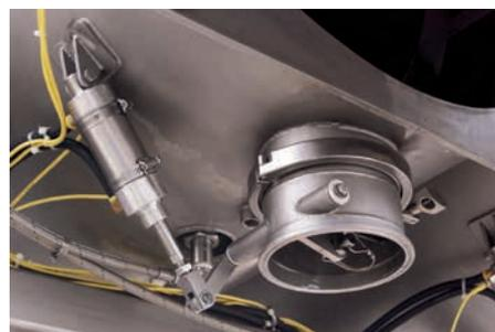
Air-operated liquid drain.
