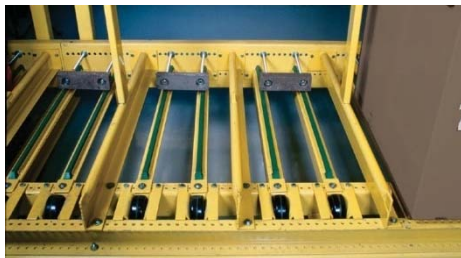
Battery compartment with adjustable back stop.
